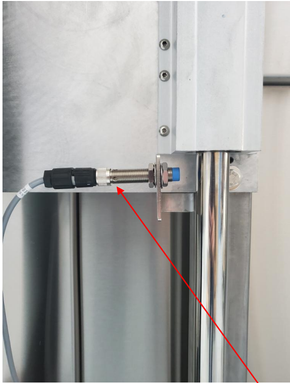
Figure 10 Lift Raised Stop Sensor
